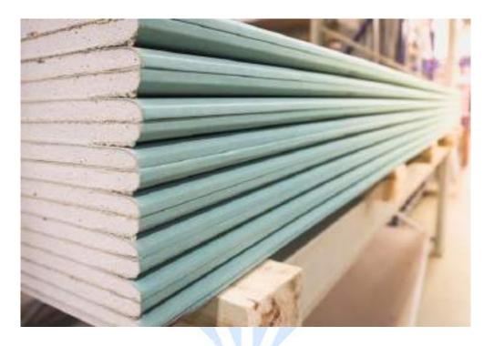
Moisture Resistant Plasterboards Consists of an aerated gypsum core with special water-repellent additives encased in and firmly bonded to, strong moisture-resistant paper liners that are green. Covered with green cardboard on face side & grey Cardboard on the back side with green edge tape. Moisture Resistance gypsum board is used as a covering material for interior walls and ceilings in residential and commercial applications that often require specific moisture or water rated assemblies.
