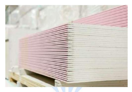
Fire Resistant Board is gypsum based interior Wall & Ceiling product used in areas where High Fire Resistance Performance is required to restrict fire to pass from one side of wall to the other side. Fire Resistant Board's gypsum core incorporates glass fibers & other fire resistive additives that are encased & firmly bonded to strong pink colored paper liners.
