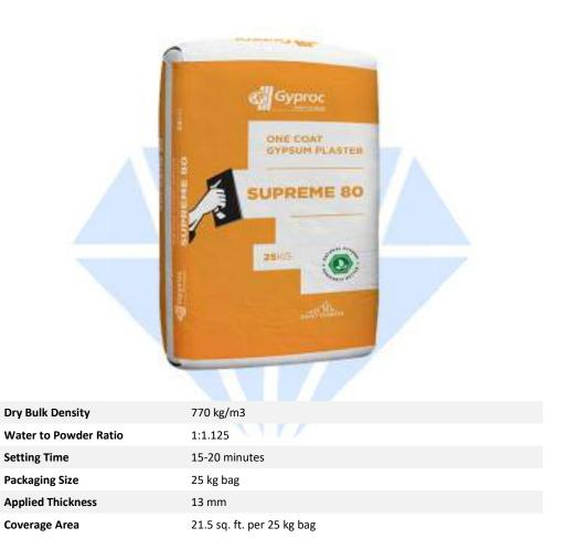
Gyproc Supreme 80 is a one coat gypsum plaster for use on almost all Internal substrates, e.g. brickwork, blocks or concrete. It provides Inert, smooth, high quality and durable base for application of decorative finishes over internal walls and ceilings. It is a lightweight, retarded hemihydrate, premixed gypsum plaster, with expanded Vermiculite aggregates, requiring only addition of clean water to prepare it for use.
