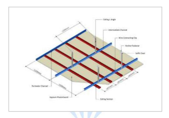
We offer a comprehensive metal ceiling framing system and accessories range to meet the challenges of modern day construction. Our range of metal framing provide basic support, strength and integrity to the false ceilings.
